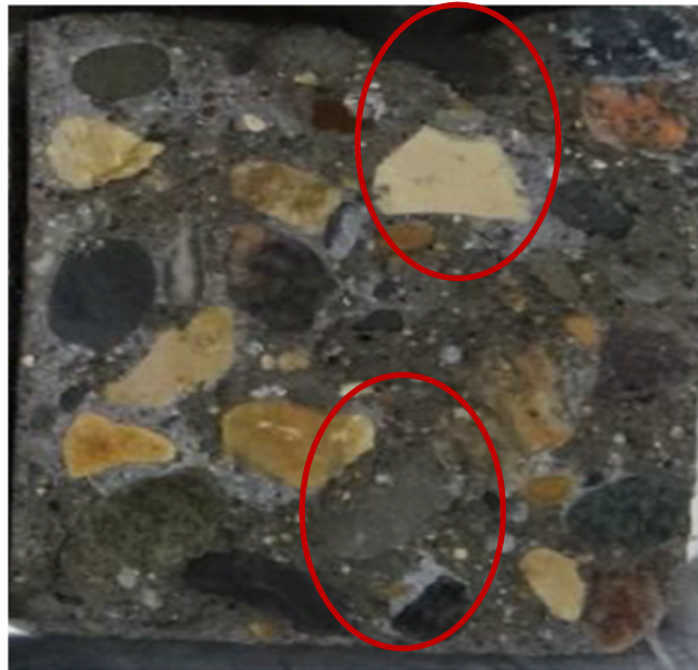
Figure 25. Sample in MgCl 2 solution after freezing and thawing (Zhang and Taylor, 2013)
