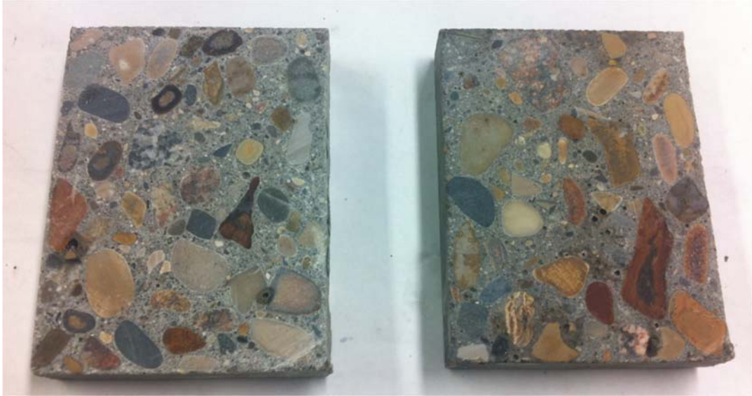
Figure 20. Concrete slices before soaking
